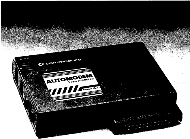
FIGURE 10-3. The Commodore AUTOMODEM.
