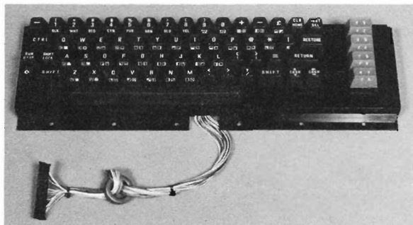
Figure 14.1. The naked keyboard.
