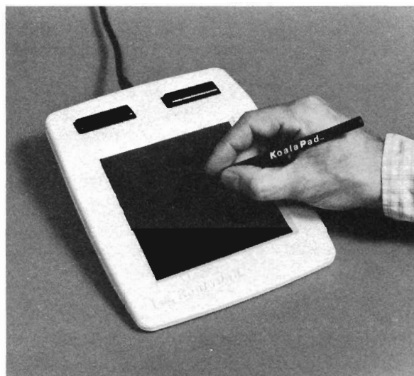
Figure 6.4. The KoalaPad is a versatile graphics input tablet.
