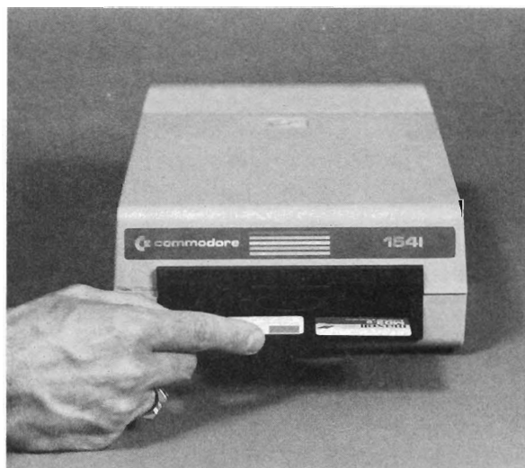
Figure 5.8. Loading a diskette
